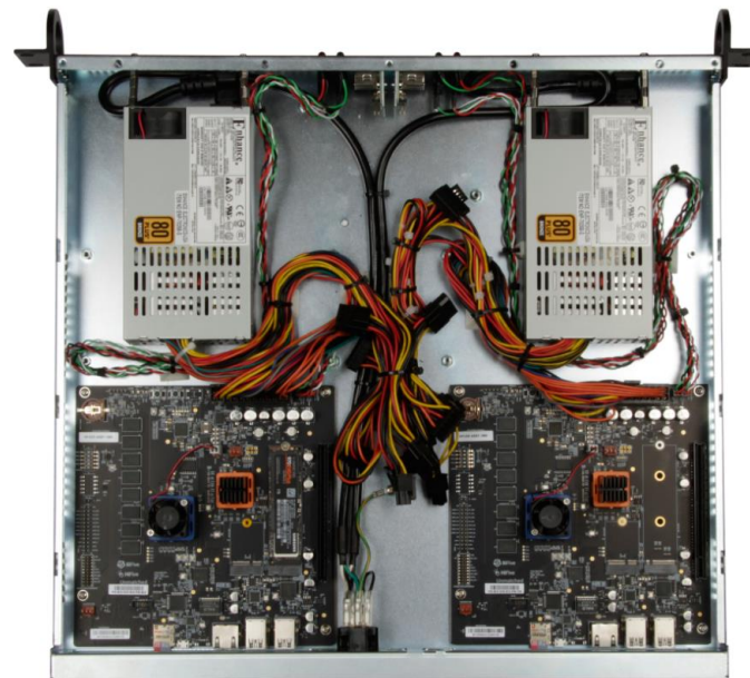
The Monte Cimone Server Blade hosts two SiFive HiFive Unmatched boards, each with a Freedom U740 SoC. It has a form factor of 4.44 cm (1 Rack-Unit) in height
